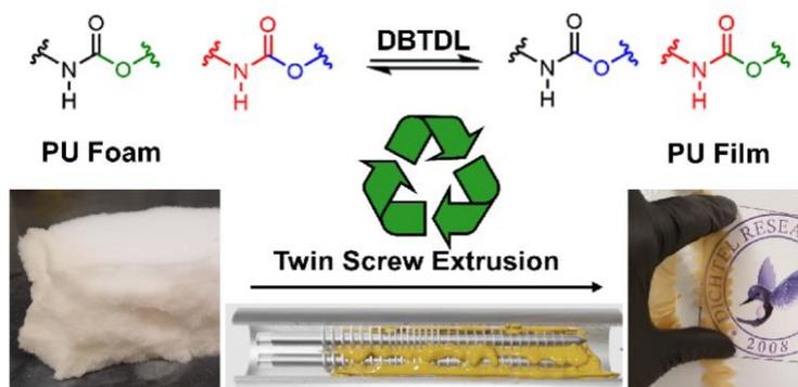
*Polyurethane foam waste is successfully reprocessed via a dissociative carbamate exchange mechanism activated at elevated temperature by a dibutyl tin dilaurate (DBTDL) catalyst with effective mixing via twin screw extrusion.*
