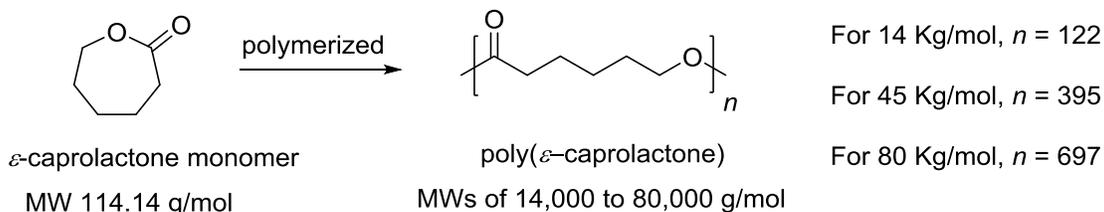
Figure 3: The  $\epsilon$ -caprolactone monomer can be polymerized to form poly( $\epsilon$ -caprolactone) polymer with varying molecular masses.
