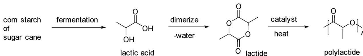
Figure 4. Steps to convert corn starch or sugar cane to polylactide, a commercially available renewable and compostable polymer.
